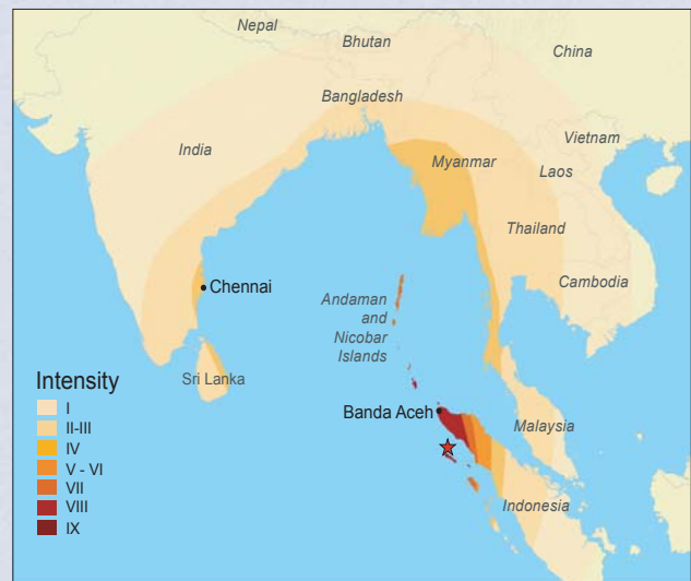
Modified Mercalli Intensity (MMI) map of the 2004 earthquake, showing violent shaking and heavy damage (MMI level IX) on the western coast of the Aceh Province of Indonesia
