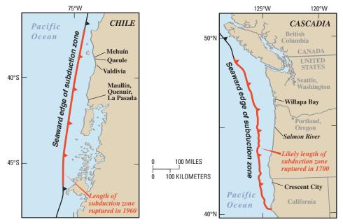
Both the 1960 Chile earthquake and the 1700 Cascadia earthquake were caused by sudden ruptures of long segments of subduction zones. Each of these quakes generated a tsunami that not only struck nearby coastal areas but also caused damage in coastal areas as far away as Japan.
